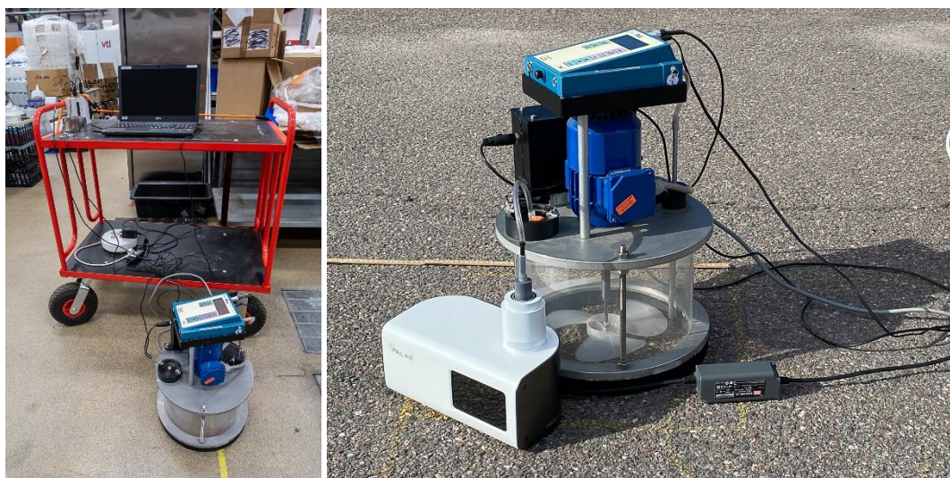
Figure 117. Duster II with wagon and computer (eft), with connected AQguard (right). Photo: Mats Gustafsson, VTi
