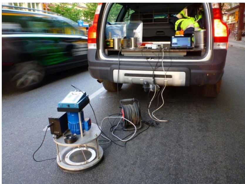
Figure 116. The original DUSTER II during measurements in Stockholm. Photo from Gustafsson et al., (2012).
