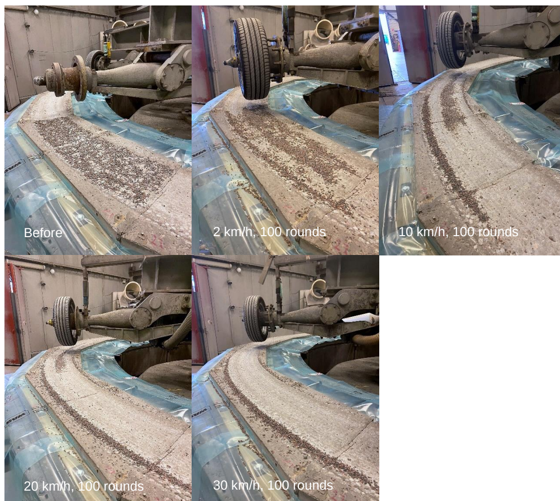
Figure 47. Applied sand on two slabs before test (left) and resulting sand distribution after test (right). Photo: Mats Gustafsson, VTI.
