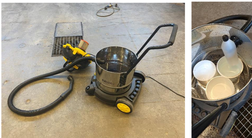
Figure 36. Vacuum cleaner used for sampling remaining sand on track. Right: modified interior to direct sample into bucket with water. Photo: Mats Gustafsson, VTi.
