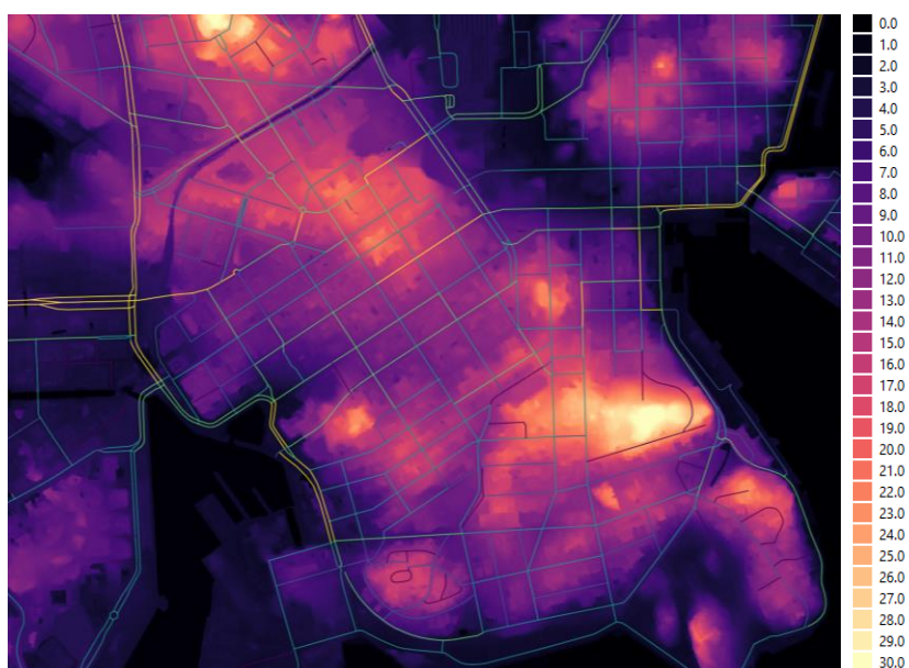
Figure 158. Detailed view of Helsinki city centre showing the 2 m resolution laser scanning surface elevation map (m) used in NORTRIP to calculate shading and long wave radiation. Also shown is the road network, as given in Figure 157
