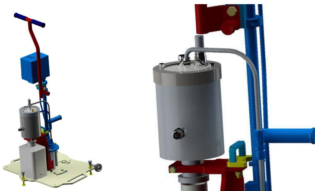
Figure 114. The WDS II designed in CAD with the direct measurement module, DMM, mounted.
