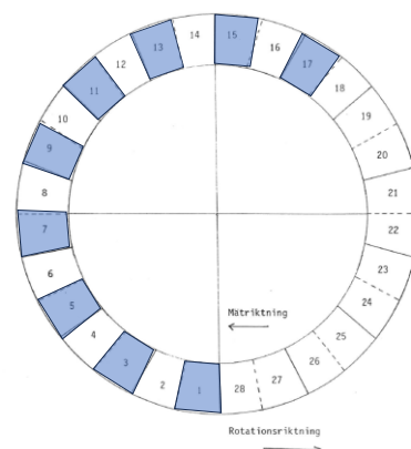
Figure 37. Pavement ring in road simulator and the used slabs in blue.
