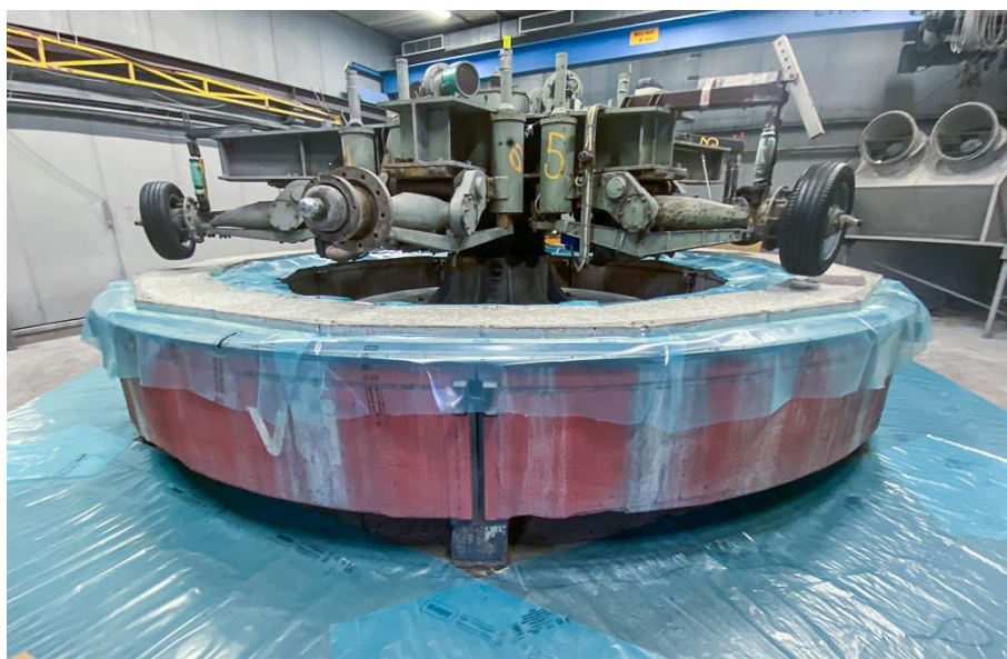
Figure 32. The VTI road simulator with plastic cover to collect sand leaving the track during tests. Photo: Mats Gustafsson, VTI.
