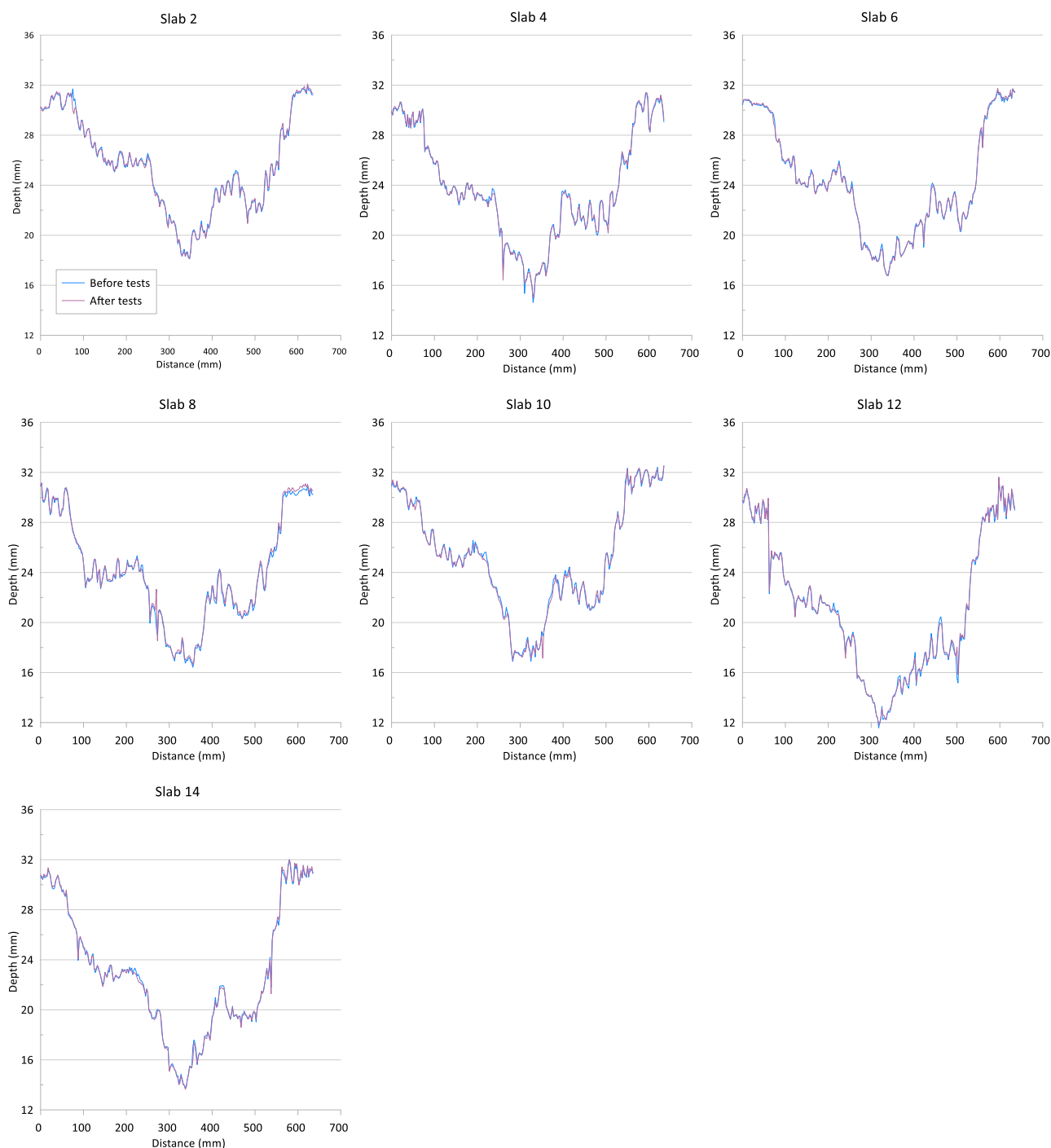
Figure 5. Profiles across seven slabs in the simulator before and after full test (all loads).
