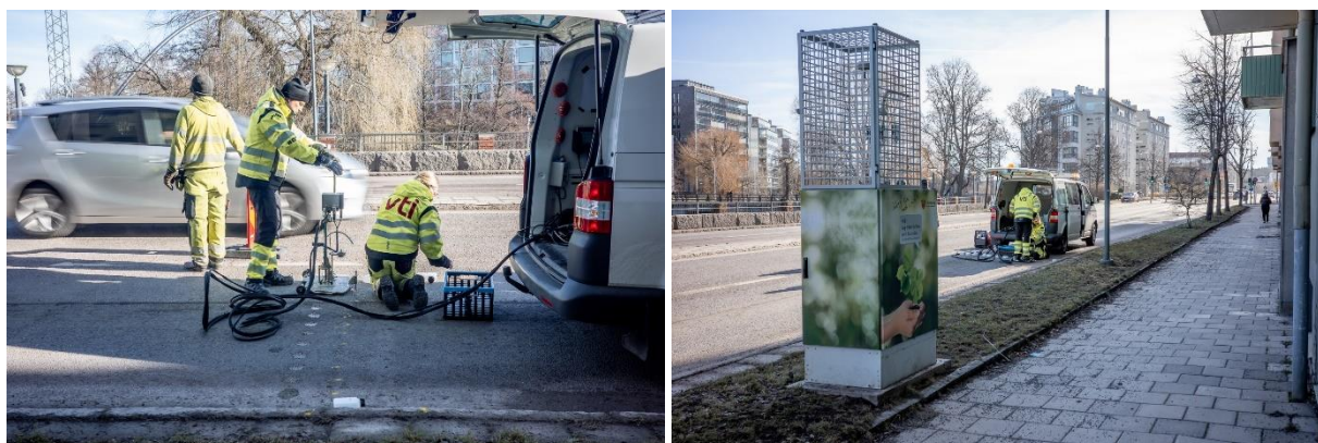
Figure 65. Field sampling of road dust and CMA with the VTI Wet Dust Sampler, WDS. Photo: Göran Blomqvist, VTI.
